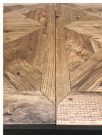
SAW MARKS (BOTTOM RIGHT) VARIENCE BETWEEN PANELS
